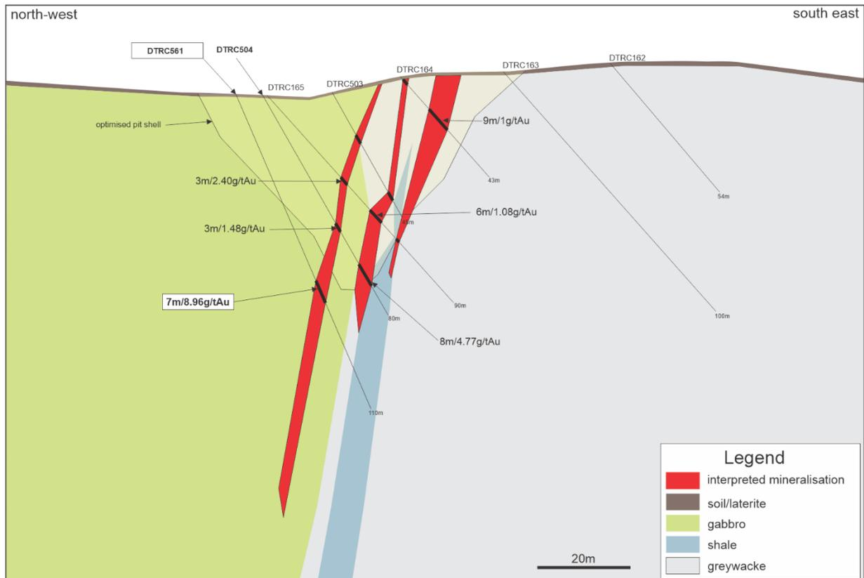
**Figure 3: Cross-section showing high grade intersection in drillhole DTRC561**
