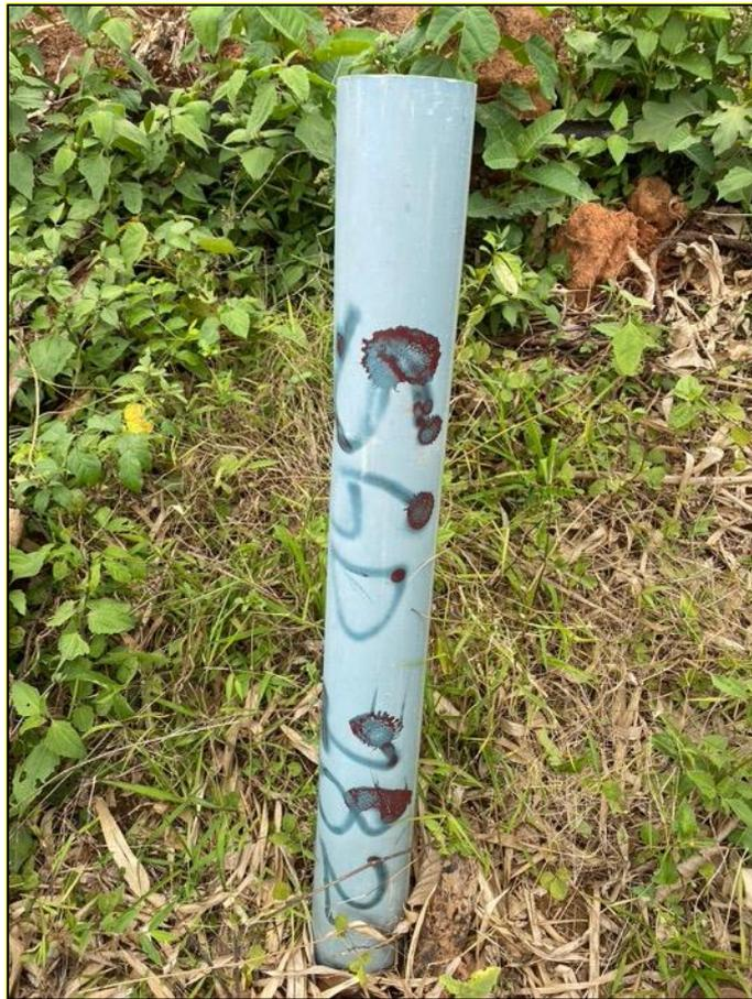
Figure 10-2. Typical drillhole collar (hole SGD 282) – blue polypipe without a concrete base (9th March 2021)
