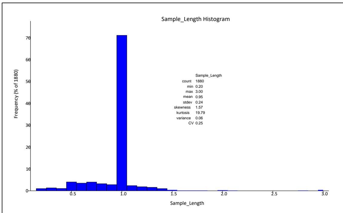
After consideration of relevant factors relating to geological setting and mining, including likely mining selectivity and bench/flitch height, a regular 1.0 m composite was selected as the most appropriate composite interval. A total of 149 samples greater than 1.0 m were split to make the 1.0 m composites. Composites of less than 1.0 m were retained by addition to the previous composite resulting in a composite file containing composites between 1.0 m and 1.7 m.
