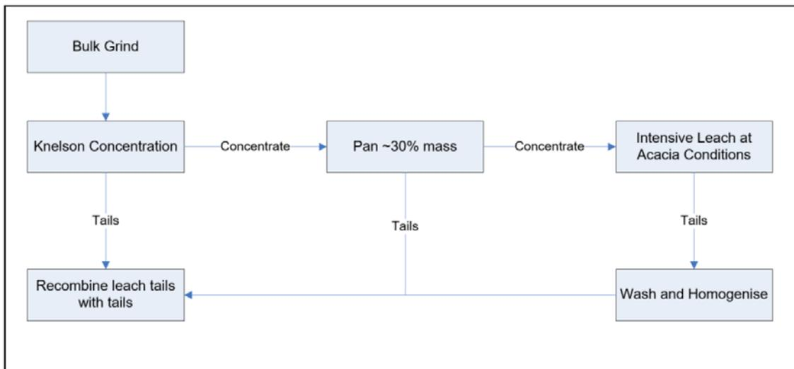
Gravity gold recovery of the variability composites presented in Tables 13-14 and 13-15 was back-calculated from the intensive leach solution assays and averages of the calculated head grades from the gravity tailings leach tests.
