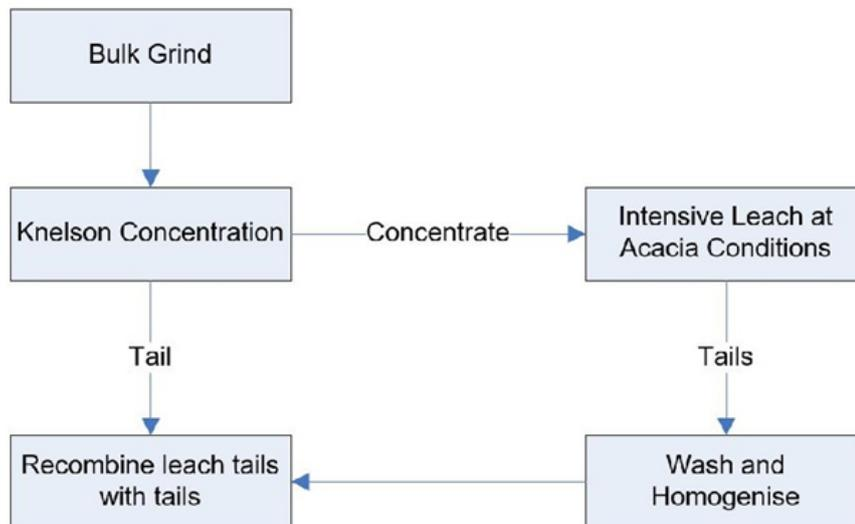
Gravity gold recovery presented in Table 13-9 was back-calculated from the intensive leach solution assays and average calculated head grades from the gravity tailings leach tests. Summarised results indicate a mass recovery of 0.48% and high gravity recoverable gold of 77.6%.
