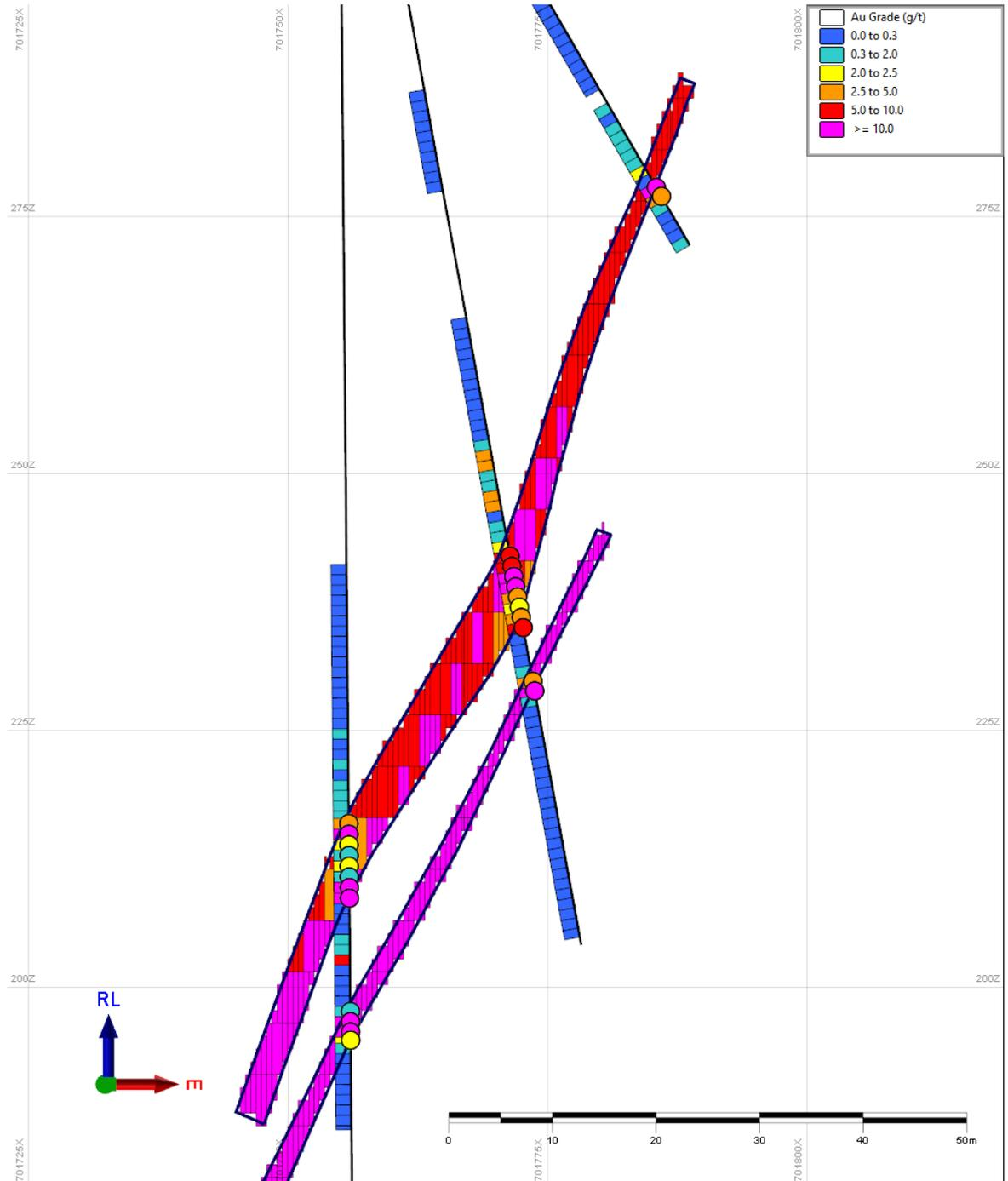
2. Volumetric comparison between the underground wireframes and the block model. The volumetric comparison check between the wireframe volume and the block model flagged with the wireframes indicates that there is a 0.24% difference between the volumes (Table 14-32). This indicates that the current block model setup is providing a good reflection of the resource wireframes.
