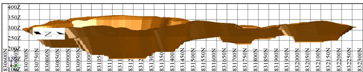
**FIGURE 15-6 DFS FINAL PIT DESIGN, 3D VIEW SHOWING INDICATED ORE  $\geq 0.77\text{G/T AU}$**
